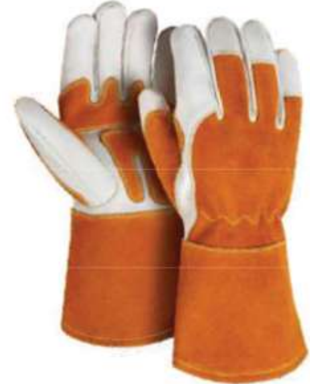
GA-TM-006 MIG Welding Gloves. Premium tan grain cowhide palm for dexterity with durable rust split cowhide back. Reverse goatskin reinforced palm and thumb. Kevlar stitching. Cotton fleece lined. 4-1/2" split cowhide cuff.
