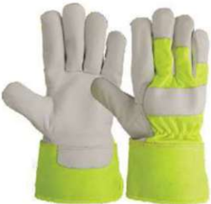
GA-CWG-007 Cow grain leather with patch palm and vein protection. Fluorescent fabric back. Lined palm. 8cm Fluorescent Cuff. Shirred Elastic Back.
