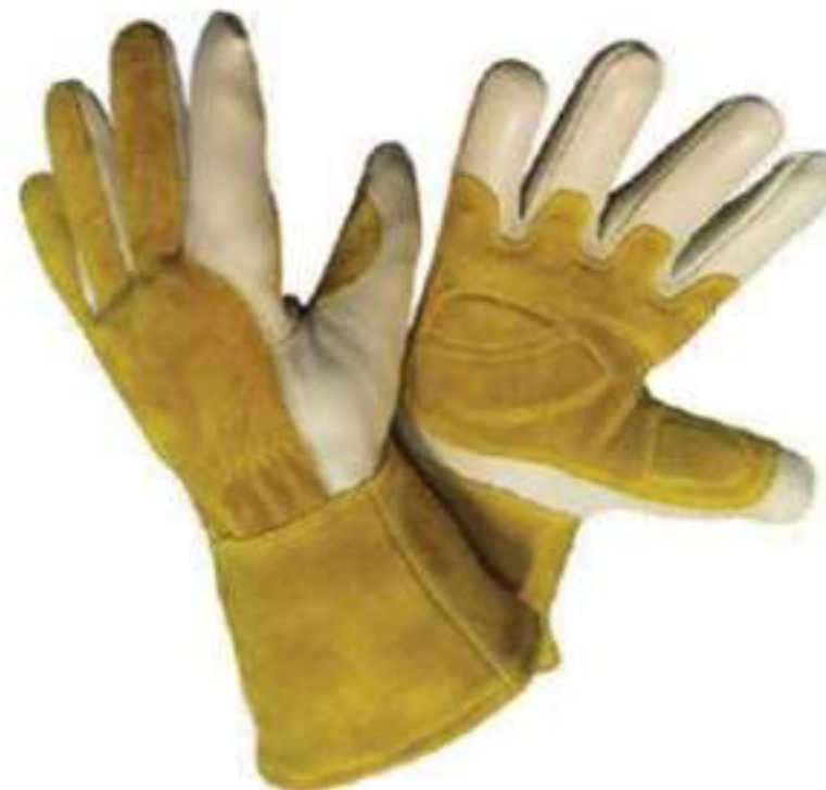
GA-TM-008 Top grain cowhide MIG welding gloves. Cowhide split reinforcements with gel padding. Cowhide split back with elastic. Fleece lined. 4" cowhide split cuff. Kevlar stitched.
