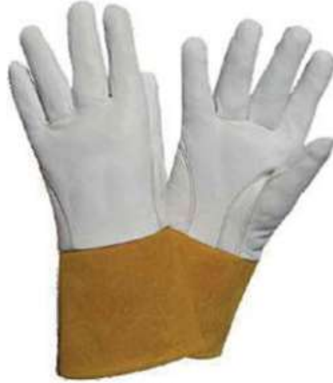
GA-TM-002 Top Grain Goatskin TIG Welding Gloves with 4" Split leather Cuff. Reinforced thumb. Kevlar stitched.
